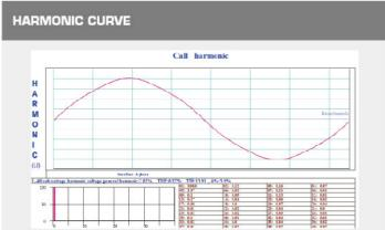
This generator tester can measure most electric parameters of a single-phase or three-phase AC generator. The standards it complied with are GB/T 2820-1997 and GB 2820-90. The signal frequency can be measured varies from 45 Hz to 65Hz. You can select one wiring mode from four modes –  $1\Phi$ 2W,  $3\Phi$ 3W,  $3\Phi$ 4W and 3V3A. The following table shows the parameters: It's the best way to replicate, prove and verify the real-life demands on critical power systems.
